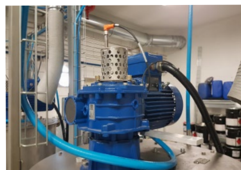
OPTIONAL FOR MIXER: Control device for speed monitoring (rpm)
