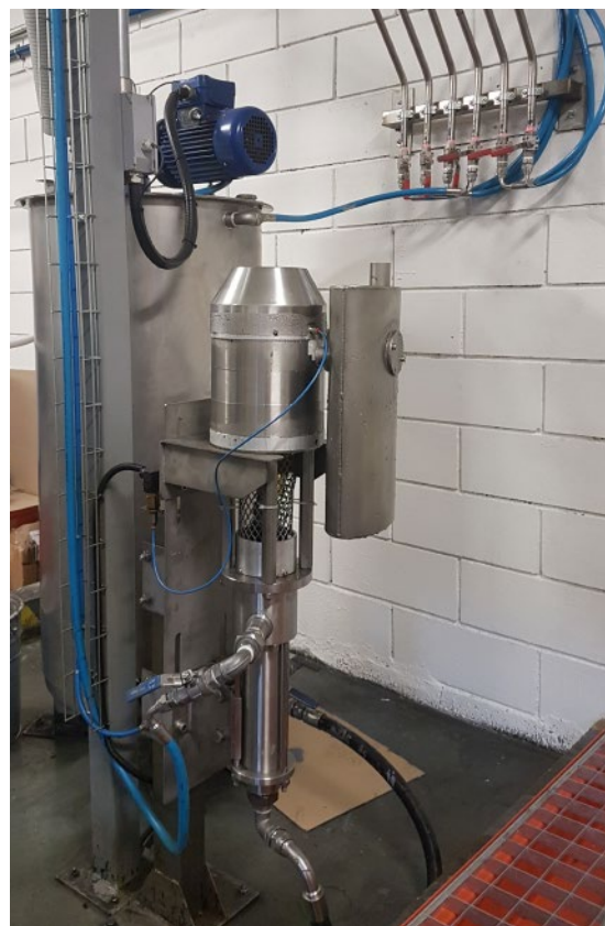
Pneumatic motor pump Airmation series 920 for centralized supply to process machines (suction phase from centralized mixing station)
